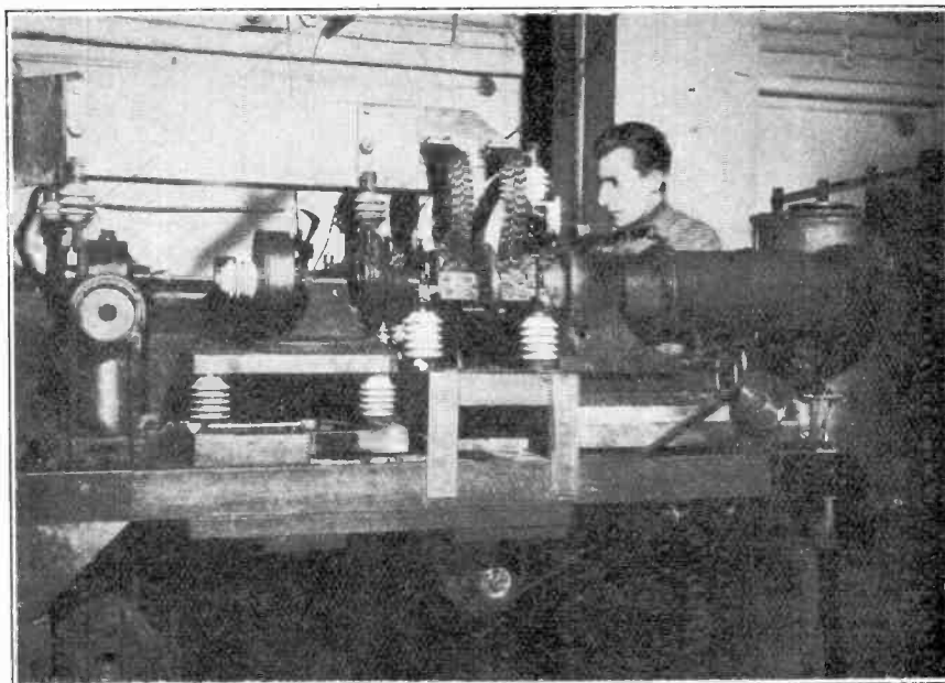
Fig. 3. The spark gap, with ventilated revolving electrodes, and arranged so that the total sparking distance is synchronously broken down by the discharge a condenser bank separate from the main oscillator.
