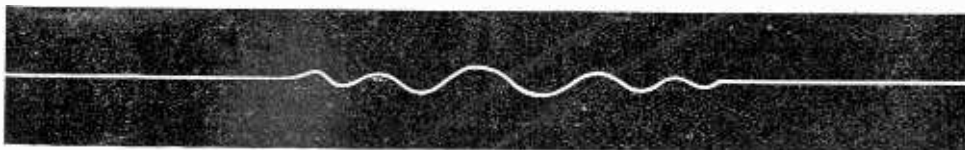
Fig. 2. The two components of a mechanical lantern slide for demonstrating wave motion. The white lines represent the transparent portions. The grid and wave line stand face to face in
